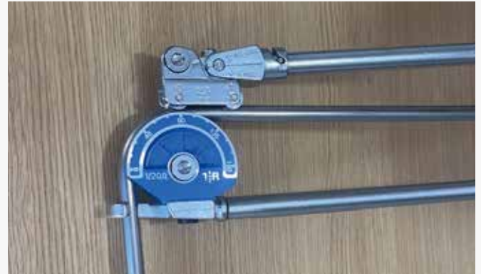
Bend the pipe with a pipe bender
